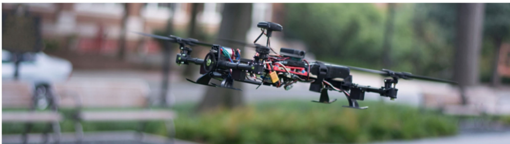
a) Autonomous, reduced-g research vehicle during an experimental flight test
